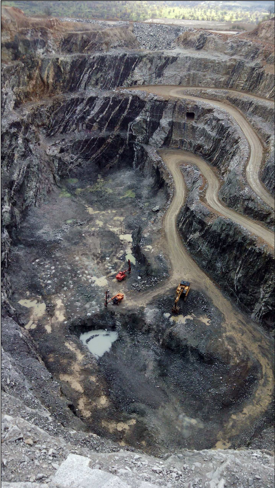
Figure 16-8. Haul Road System at Los Santos Sur
