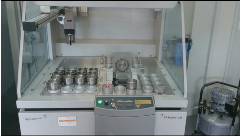
Figure 11-5. On-Site AXIOS XRF Assaying Equipment
