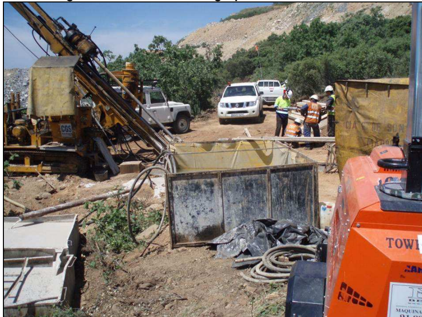
Figure 9-1. Diamond Drilling Operations at Los Santos
