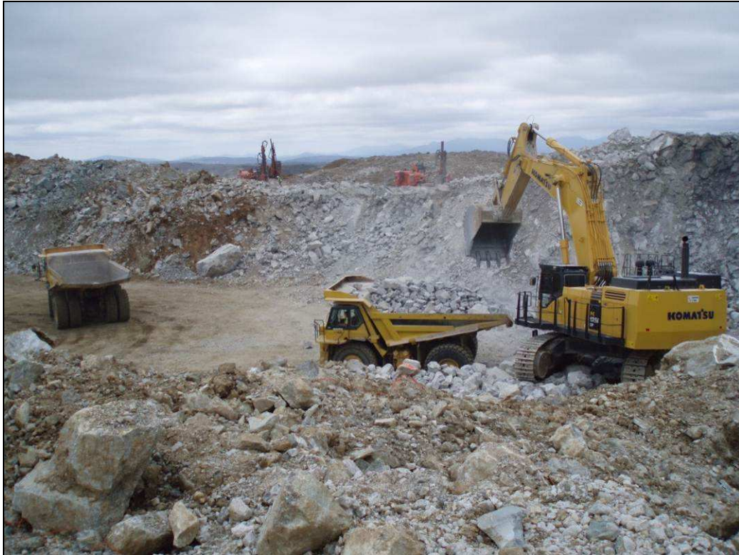
Figure 16-4. Mucking Operations at Los Santos Sur
