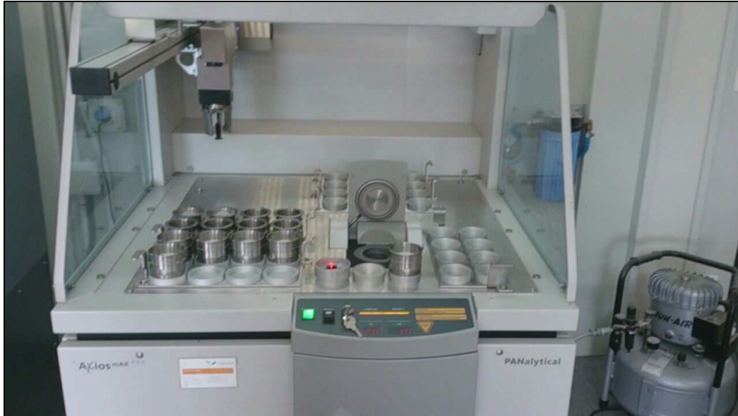
Figure 11-5. On-Site AXIOS XRF Assaying Equipment
